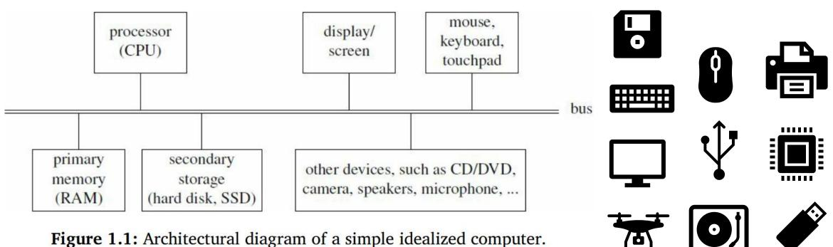
Figure 1.1: Architectural diagram of a simple idealized computer.
